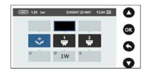
4) At the end of the washing cycle, the continuos buttons will start flashing again and it will be possible to activate the rinse cycle. Before and during rinsing, the machine indicates the chosen group number + R; as long as the rinsing procedure is not carried out entirely, the group is blocked.
